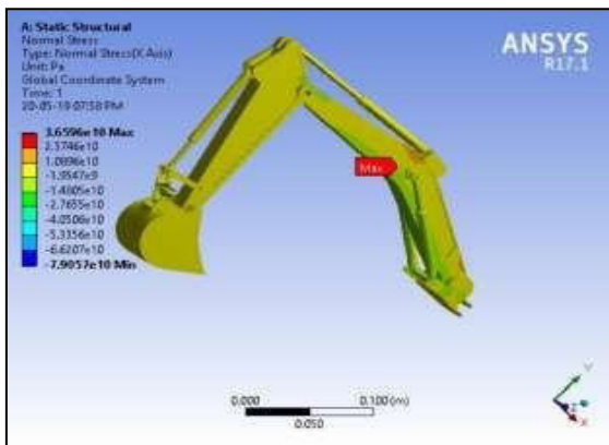
Fig. 3: results of analysis of excavator arm without vibration
