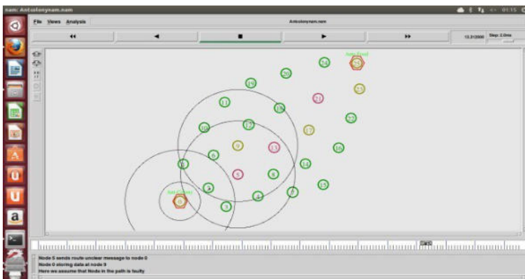
Fig.2 the forward ants are forwarded towards the food source. The routing is taking place.
