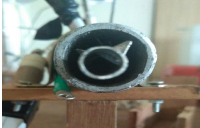
Figure 8 f Pipe with Triangular Fin Insert in Test Section
