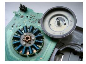
Fig. 1- fig shows the BLDC motor used in floppy disc drive in computer.
